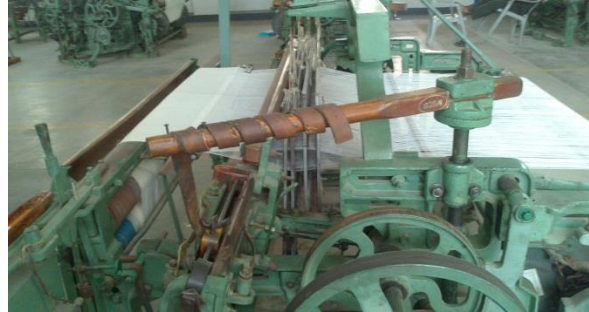
Figure 4: picking arm to be replaced by electromagnetic launcher
