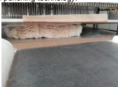
Figure 3: Process of Needle Punching
