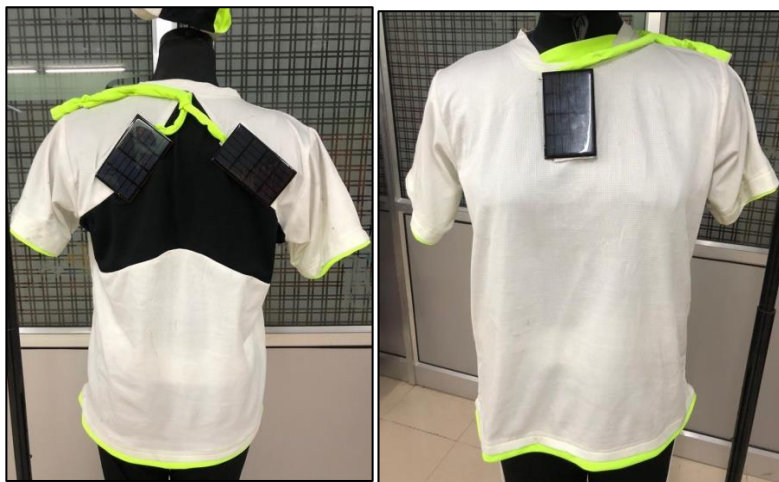
Figure 12- Solar panel integrated t-shirt
