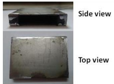
Figure. 1 Mould dimension for fibre pull out test (10mm width, 50mm breath and 70mm height)
