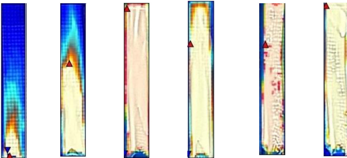
Figure 3: Thermal image of Sample 2 at different burning time
