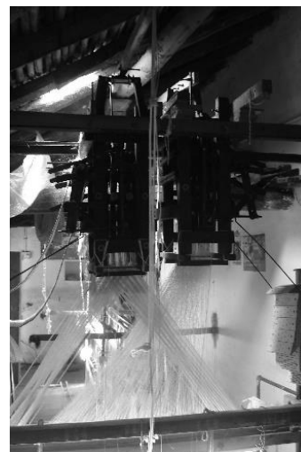
Figure 2. Multiple jacquard system fitted above a throw shuttle pit loom
