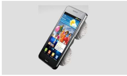
Figure 6: Smartphone airbag system [11]
