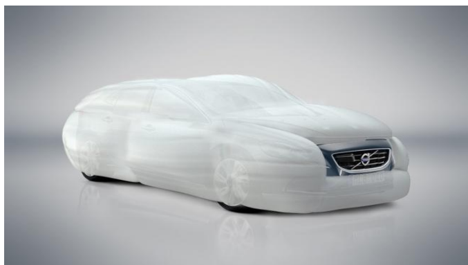
Figure 5. Volvo V40 air bag External Vehicle Protection system [10]
