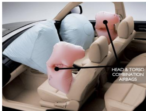
Side head and torso airbag
