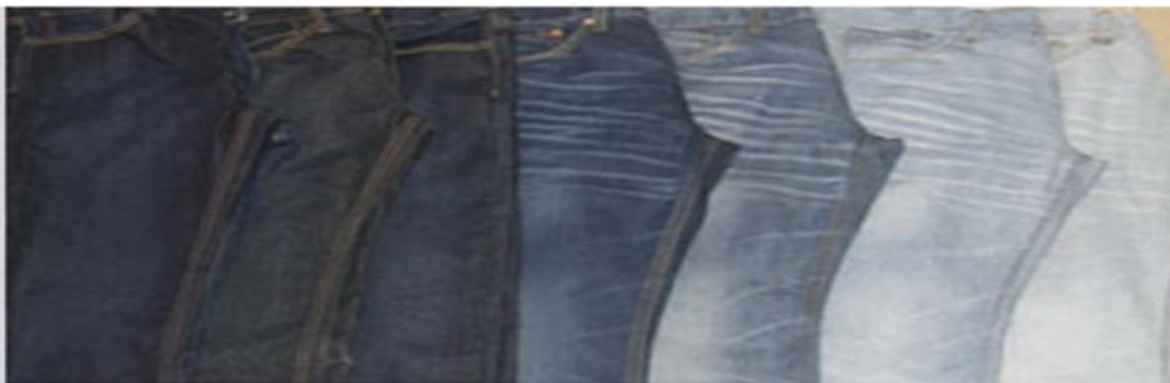
Figure 5: Range of Bleach down on Jeans with ozone finishing (Ozone Denim Systems).
