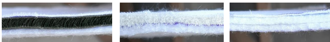
Figure 2.1 Schematic of the layers of the composite footwear insole. Figure 2.1(a) variant 1 Figure 2.1(b) variant 2 Figure 2.1(c) variant 3
